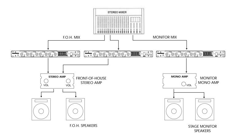
NOTE: Insert any processors, EQ's, etc. between the mixer and the FS-4N. The Feedback Suppressor should be the last processor in line before connecting the audio to the amplifier.
